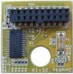
The following is the pin assignment of TPM, it uses LPC to communication with external micro controller.
