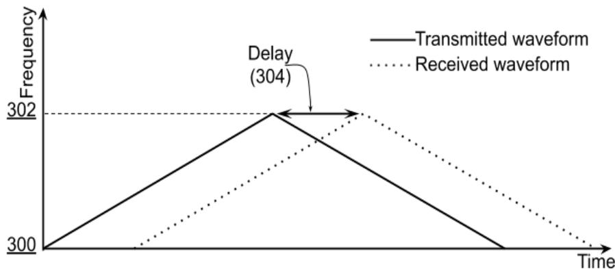
**Fig. 3: A chirp signal**
