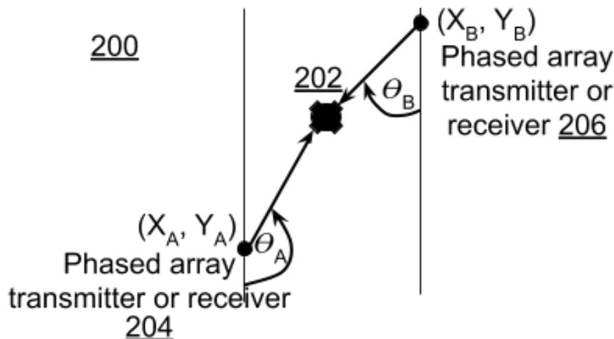
**Fig. 2: WiFi or Bluetooth phased arrays to locate objects**
