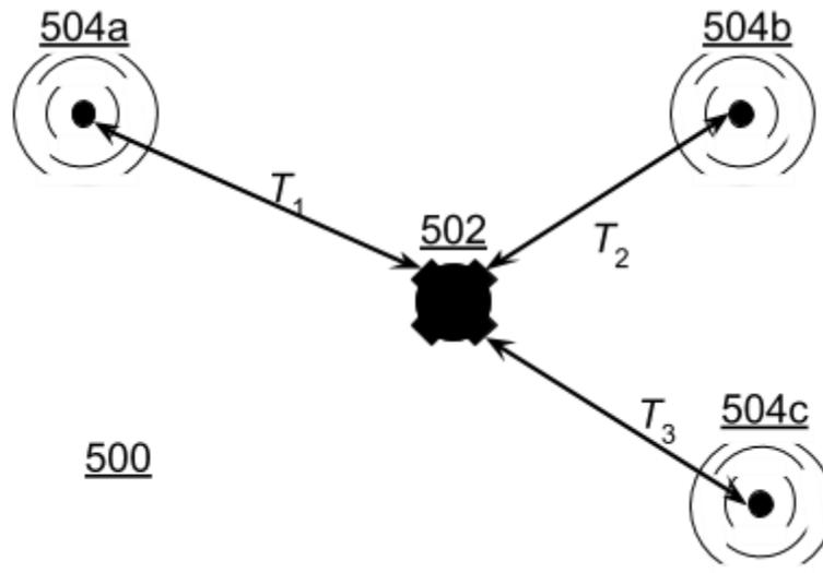
**Fig. 5: Object location using WiFi or Bluetooth chirps**
