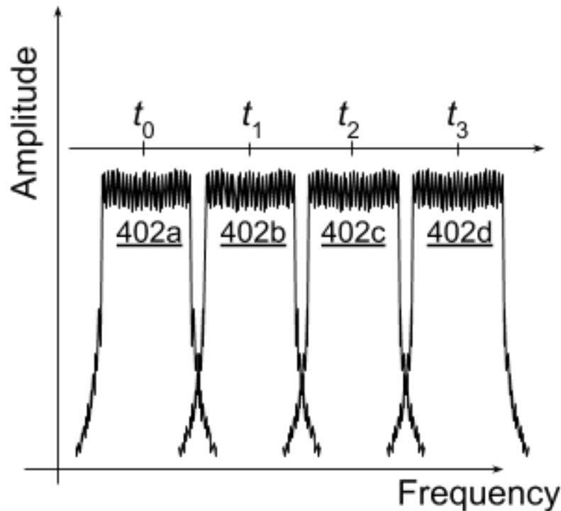
**Fig. 4: Generating a chirped WiFi signal**
