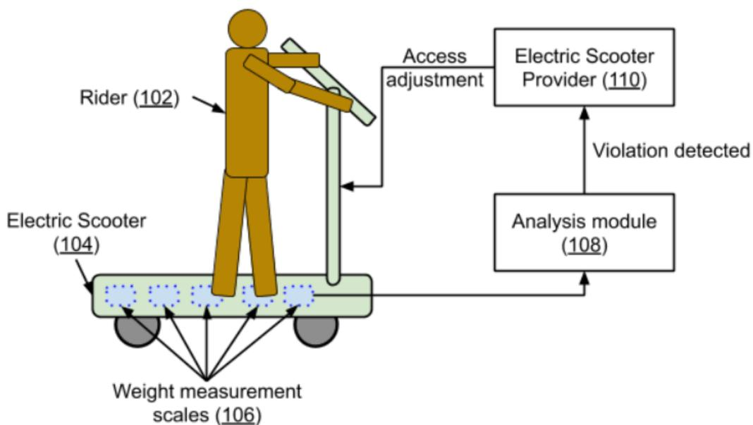
**Fig. 1: Using weight measurement scales to detect electric scooter riding behavior**
