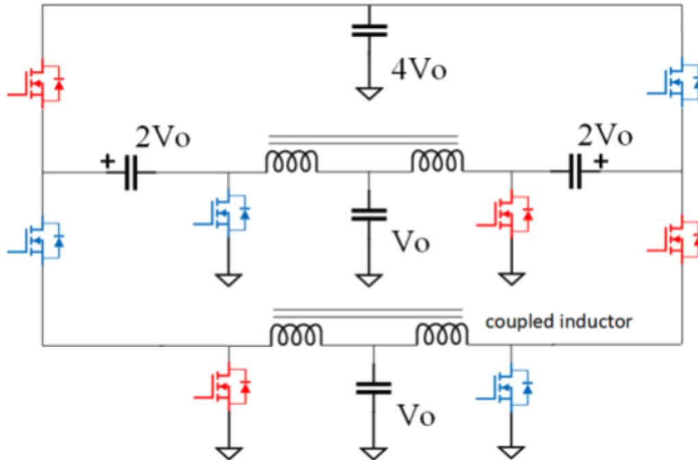
**Fig. 2: A 4:1 DC-DC converter**
