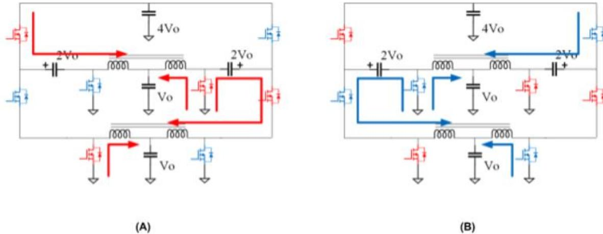
**Fig. 3: Operating stages of a 4:1 DC-DC converter (A) Stage-1 - the red switches are closed and the blue switches are open (B) Stage-2 - the red switches are open and the blue switches are closed.**
