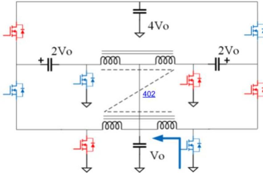
**Fig. 4: A 4:1 DC-DC converter of interleaved STC design, with a four-winding coupled inductor**
