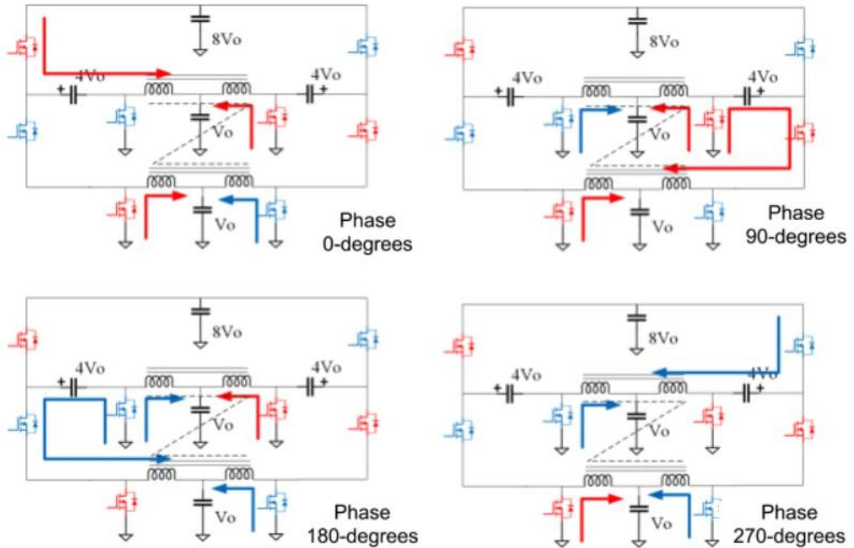
**Fig. 6: Operating stages of an 8:1 DC-DC converter constructed with a topology similar to that of a 4:1 DC-DC converter**
