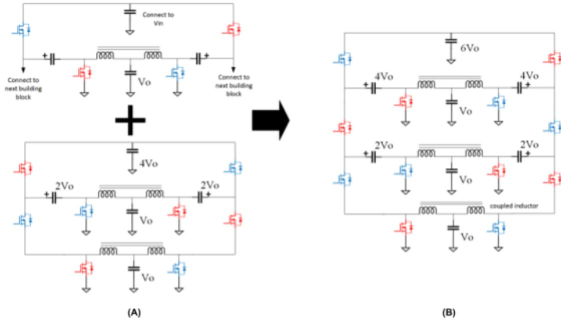
**Fig. 5: A 6:1 DC-DC converter (A) Construction from modular building blocks (B) A 6:1 DC-DC converter**
