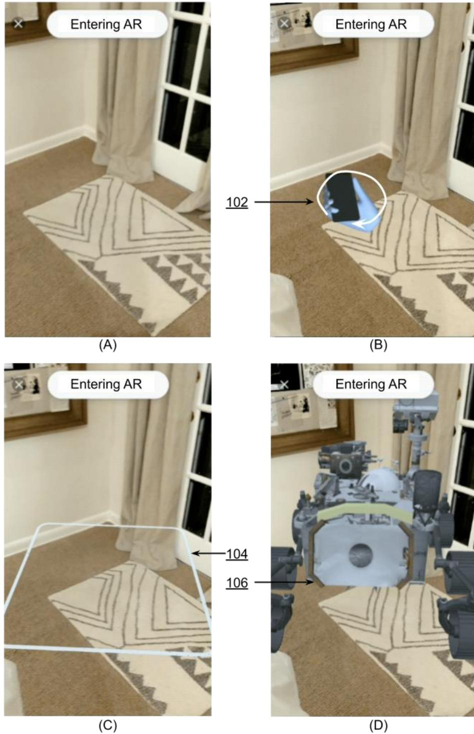
**Fig. 1: Requesting the user to move mobile device to establish correct orientation of virtual object**
