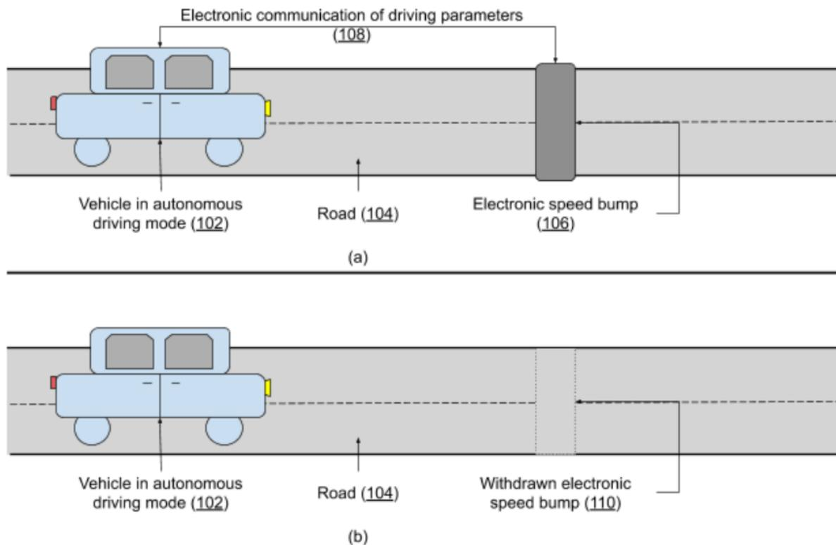
**Fig. 1: Operation of an electronic speed bump for vehicle in autonomous driving mode**
