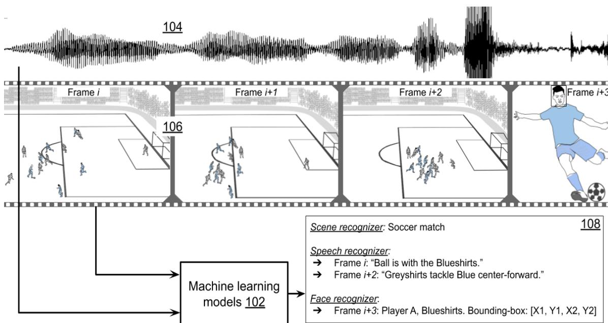
**Fig. 1: Video annotation using machine learning models to produce granular metadata**
