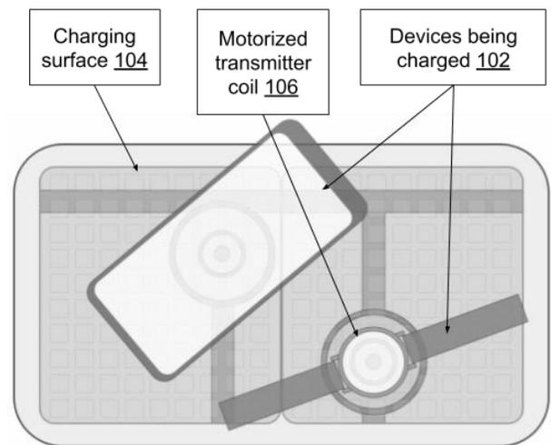
**Fig. 1: Motorized coil wireless charger with traditional alignment mechanism**
