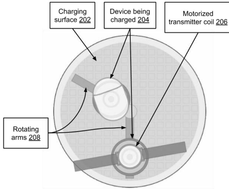
**Fig. 2: Motorized coil wireless charger with novel alignment mechanism**
