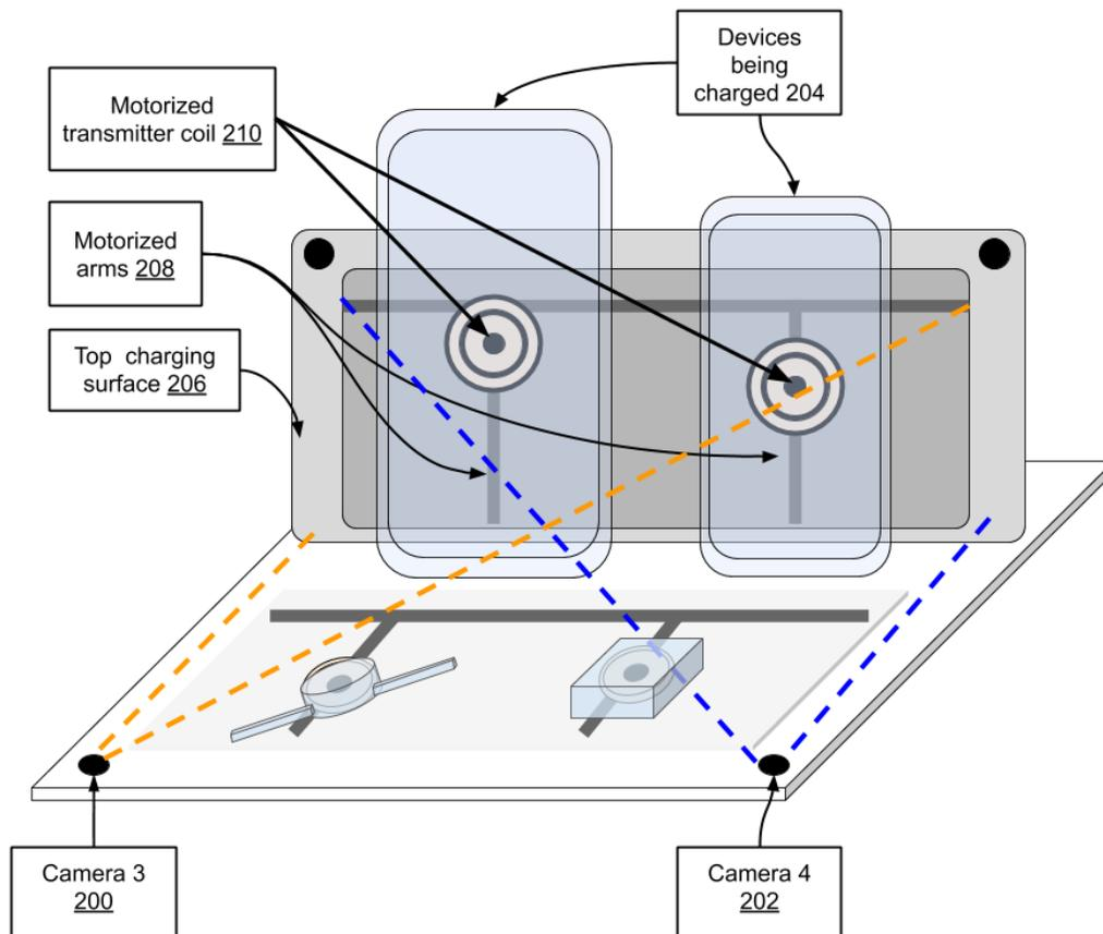
**Fig. 2: Motorized coil wireless charger with computer vision assisted alignment for top charging surface**
