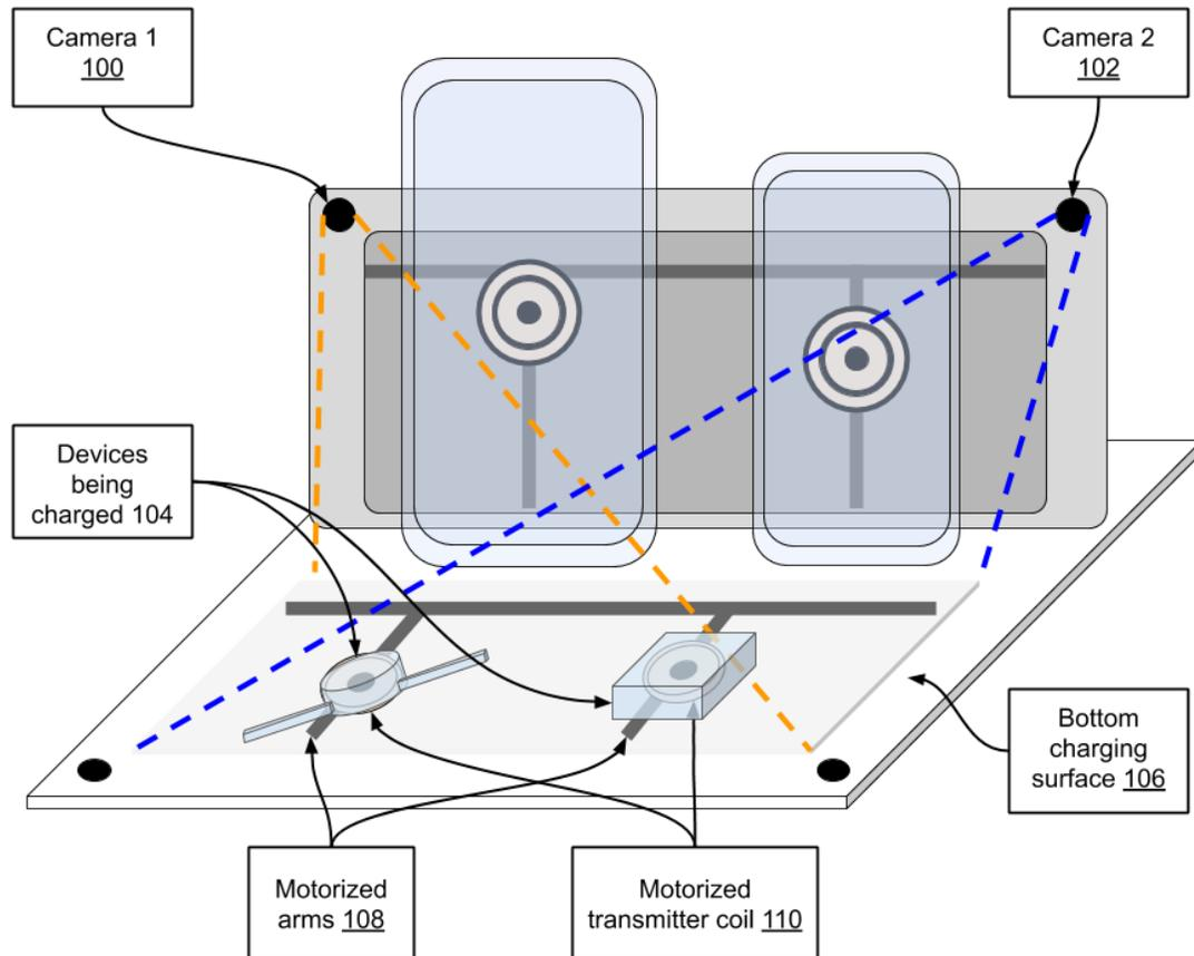
**Fig. 1: Motorized coil wireless charger with computer vision assisted alignment for bottom charging surface**
