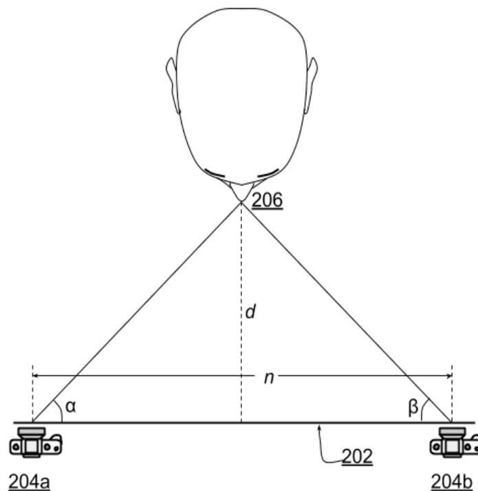
**Fig. 2: Determining the distance of a body part from the screen of a laptop or desktop**
