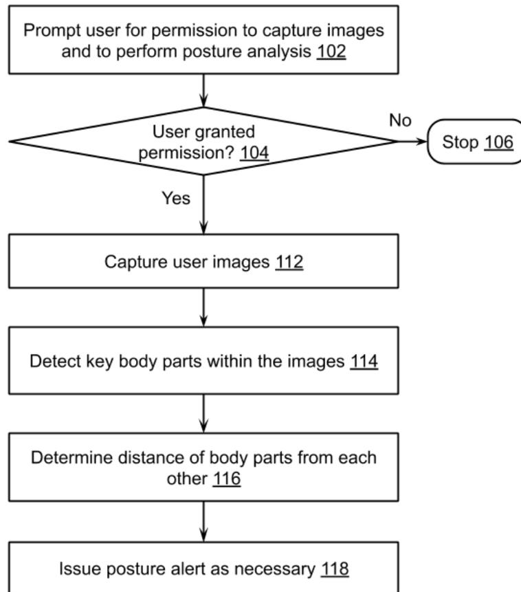
**Fig. 1: Determining posture of a user using an array of cameras**
