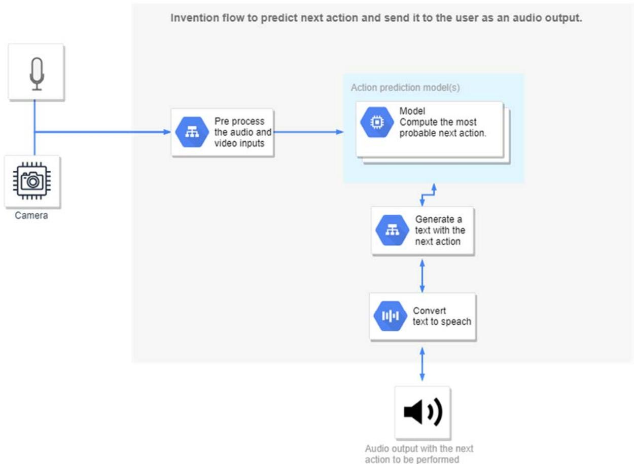
*Figure 2 - Description of the dataflow and how the prediction model is integrated in the flow.*
