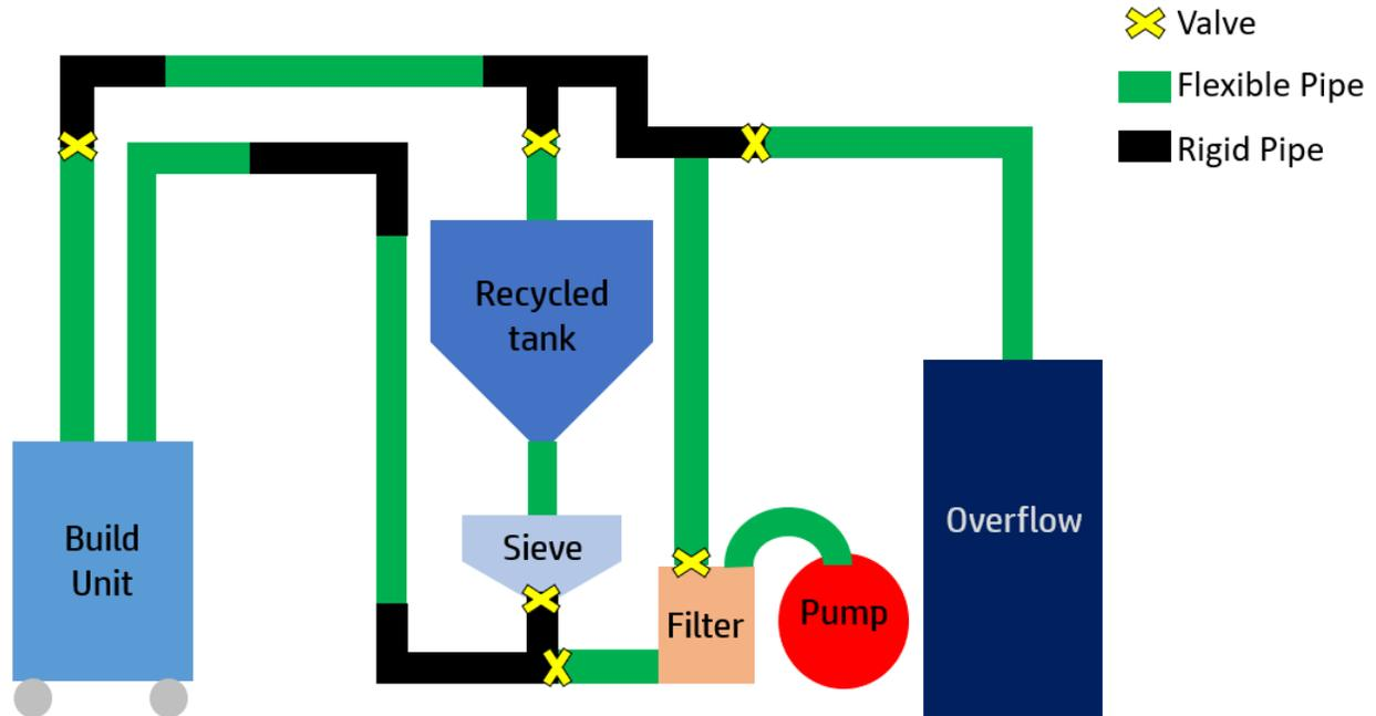
The current issue that this disclosure is trying to solve is what is shown in the illustration below. After loading and unloading processes and transporting powder through the different circuits of the units, remaining of the material can be stuck at some points and sometimes the airflow generated by the vacuum pump may not be enough to remove it and make it go to the desired volume.
