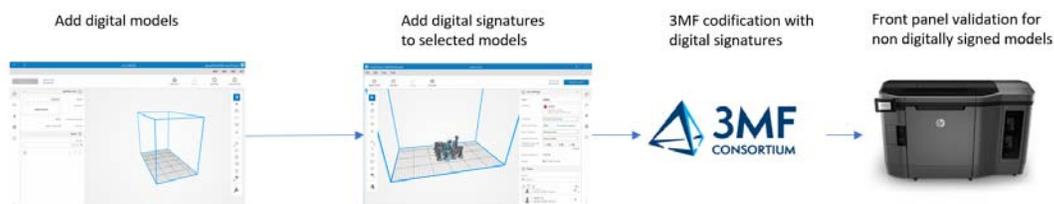
Figure 1. Standard workflow for models/jobs with digital signatures.
