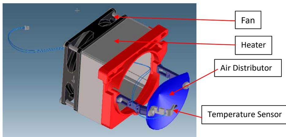
Compared with typical dryer we have added the air distributor and the temperature sensor:
