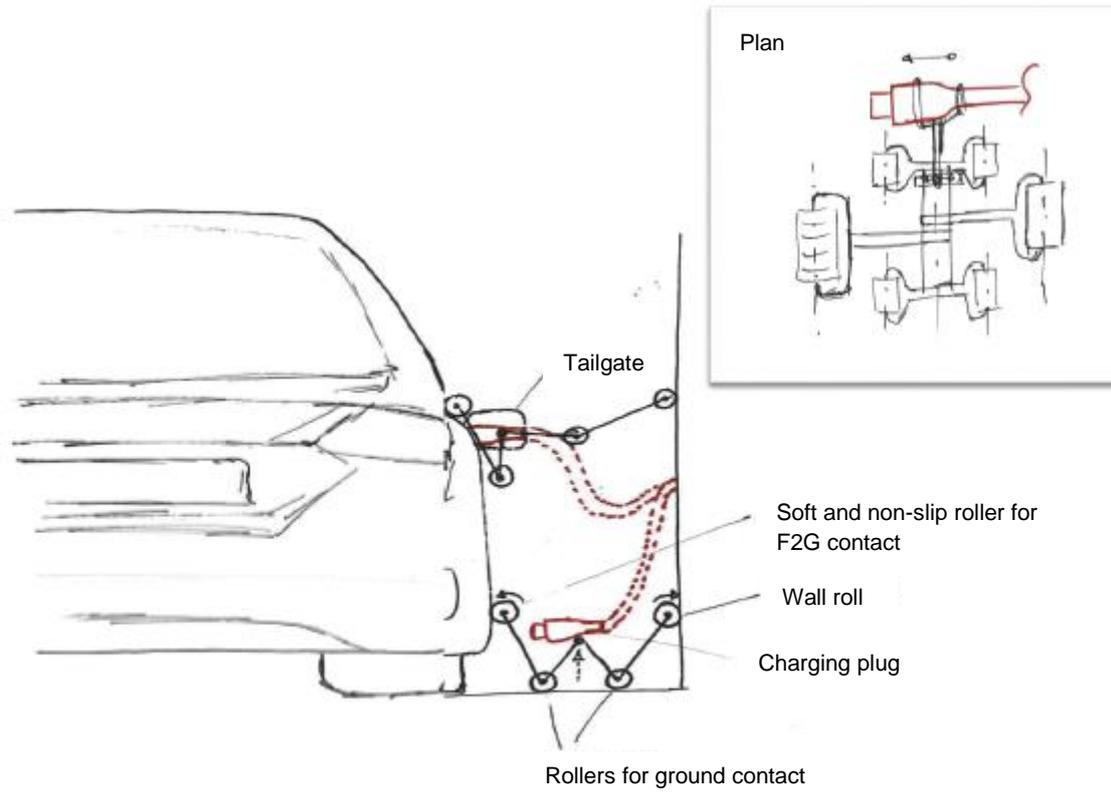
**Figure 1:** Schematic representation of minimally invasive loading robot
