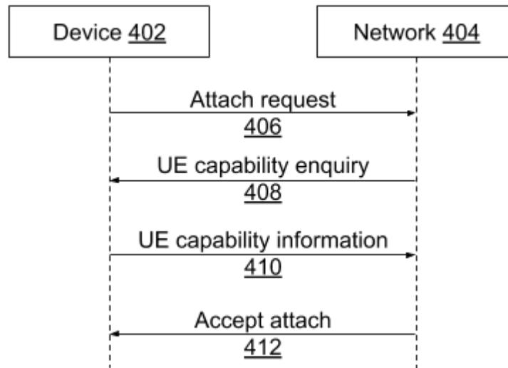
**Fig. 4: Device-network messaging to communicate UE capability**
