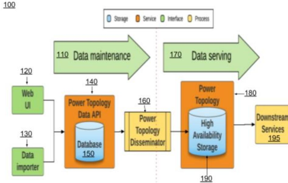
**Fig.1: Example system for maintenance and visualization of electrical power topologies**
