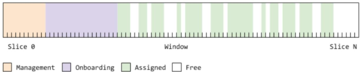
Each member can use the management slices in order to establish the timing of each slice within the window as well as when the next management slices will be sent. This allows the member to then sleep until its assigned slice when it can wake up and transmit a single packet.
