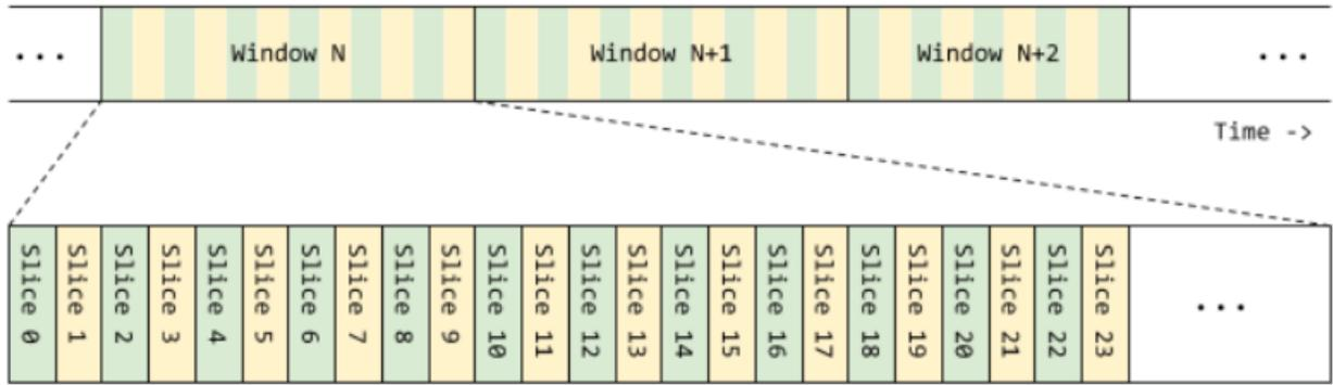
Each slice is long enough to allow a single BLE advertising packet with margin on both sides. Each window is long enough for every member using that channel to get a slice with some extra slices allocated to the management system.
