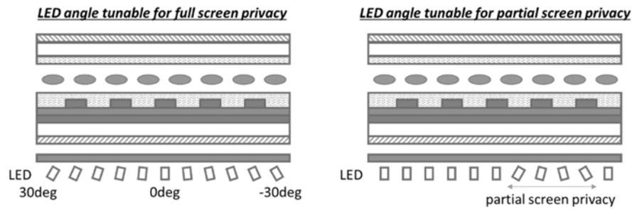
**Figure 1.** Cross section of the proposed display with angle adjustable LED. (Left) The display showing full screen privacy with all LEDs rotate toward the center of the screen, (right) the display showing partial screen privacy with LEDs in selective area rotate toward the center of the selective area.
