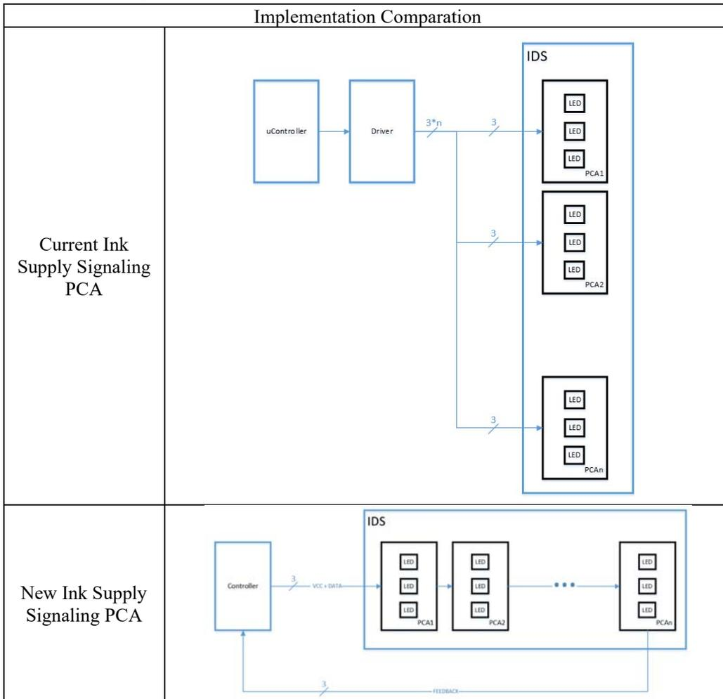
The implementation uses a simple 3 wire cable (power supply, communication and ground) to connect all the system having the possibility of connecting a feedback wire to improve the testability. The cost of the system will be improved as well as the simplicity to manufacture the printer. Serviceability will be easier.
