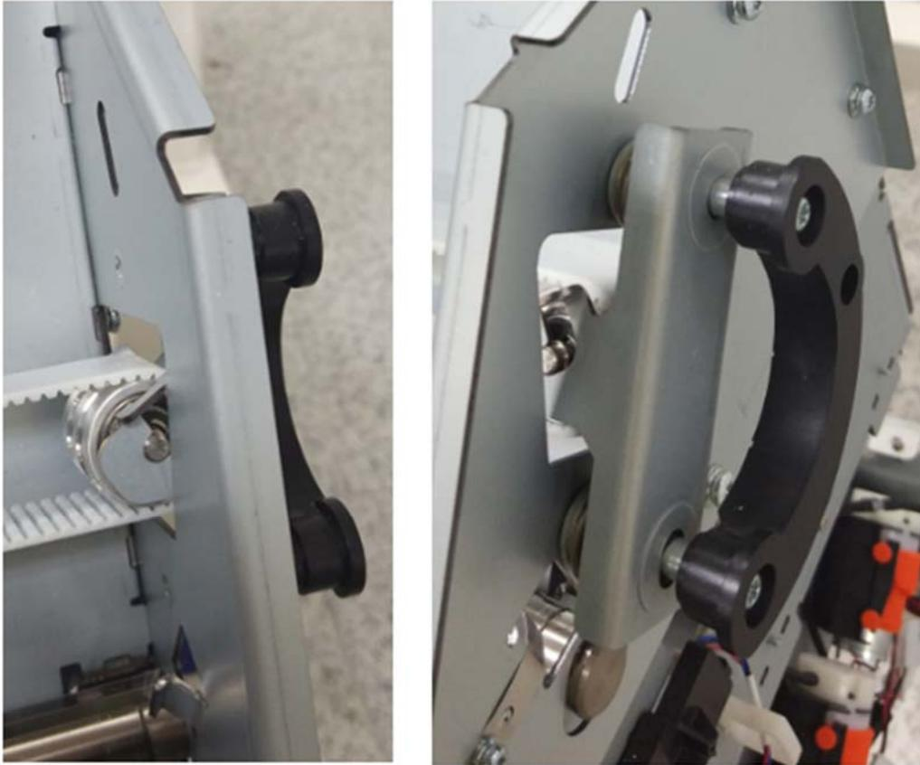
This is an image of a prototype once it is build and tensioning the belt. If we want to remove the tension of the belt for any reason we only must unscrew the black part (galgue) and screw it flipped 180°. Due to the geometry explained above once we screwed the sheet metal which is holding the pulley moves forward and the tension is removed..
