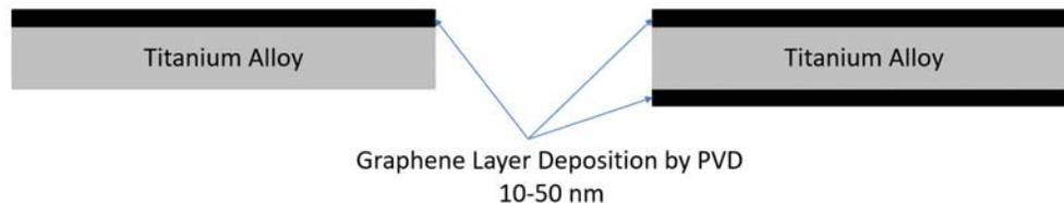
**Figure 1.** Graphene Layer Deposition on Titanium Alloy by PVD
