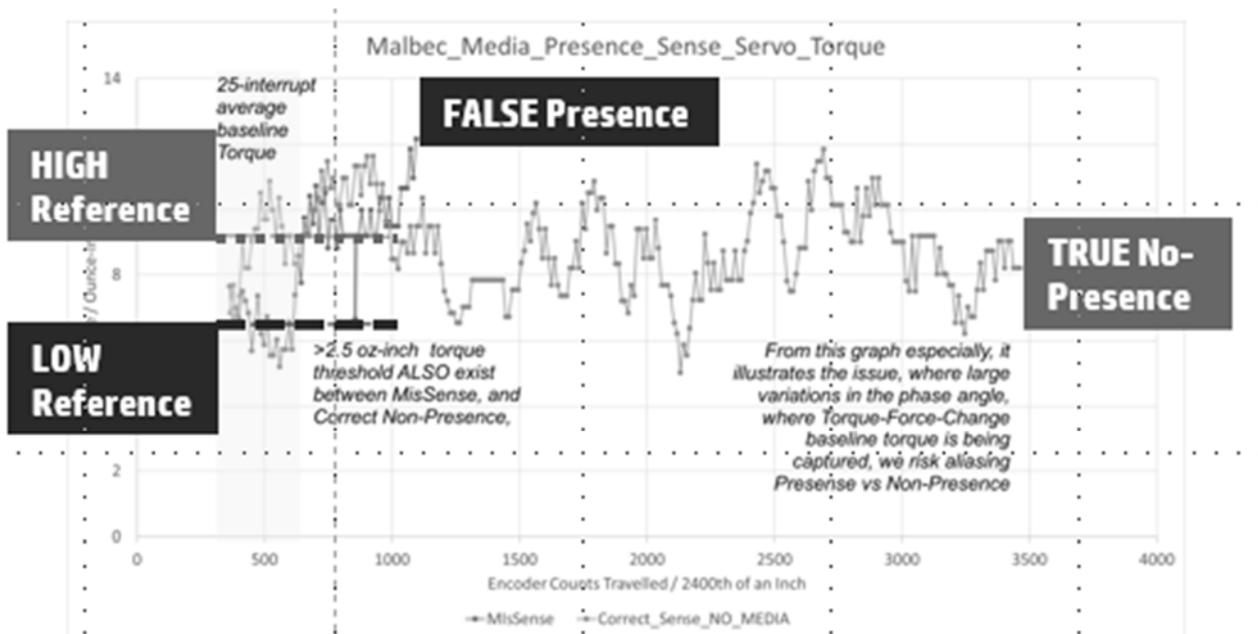
Figure 4: Difference in Capture Reference results in a very different response to trigger
