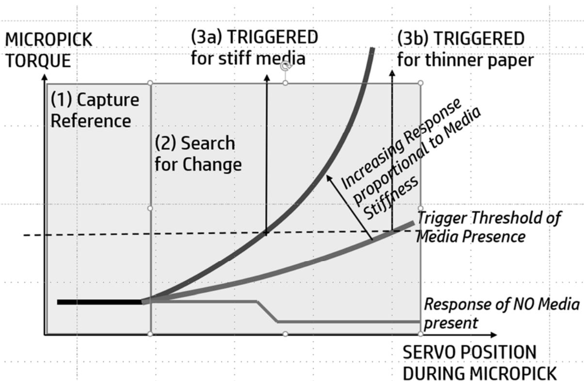
Figure 2: Step by Step description of SENSE algorithm using Torque Change, Step by step from (1) to (3)
