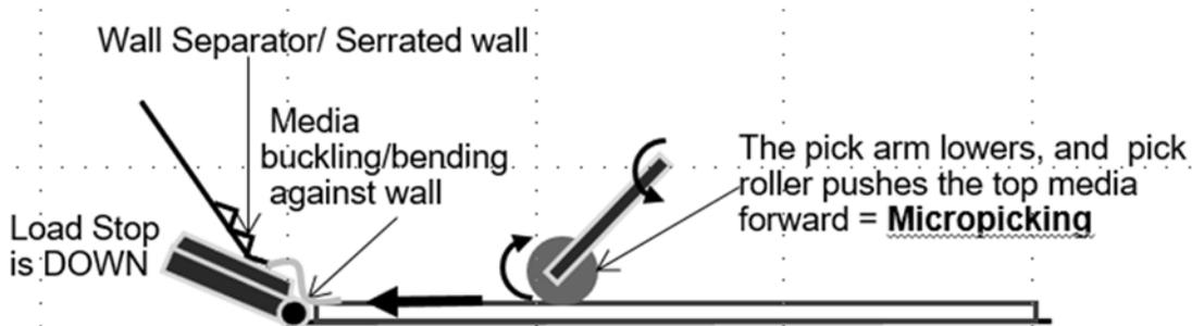
Figure 1: Example of application – Micropicking senses resistance of media against wall
