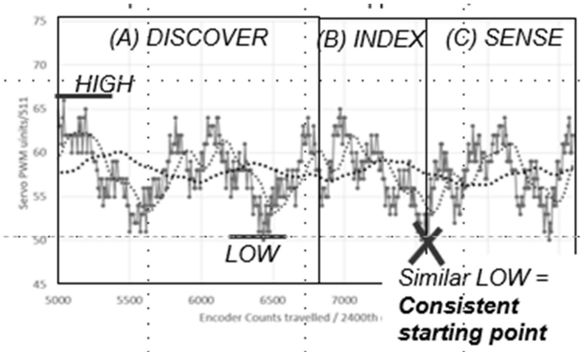
Figure 5: Adding additional Indexing actions (DISCOVER-> INDEX), before the basic SENSEmove
