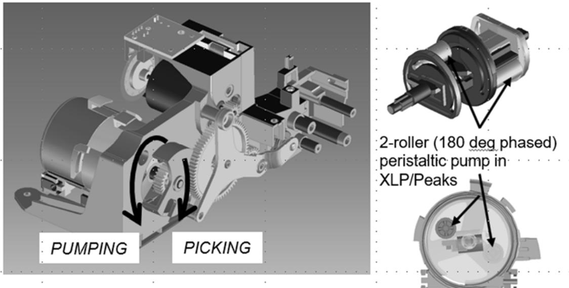
Figure 3: Shared Pick/Pump Drive system, with Pump creating a 2/rev parasitic periodic noise onto torque during picking
