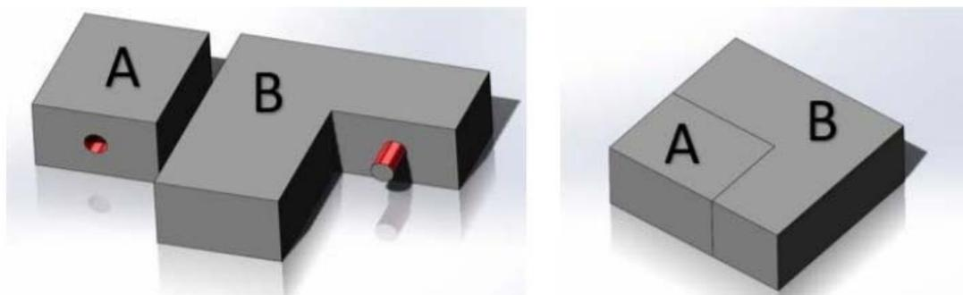
Figure 2 Color codes can also be used to mark parts that need to be assembled
