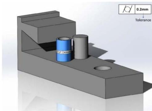
Figure 2: Dimensional tolerances could use different color codes
