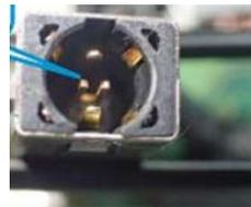
Figure 2 – damaged DC jack
