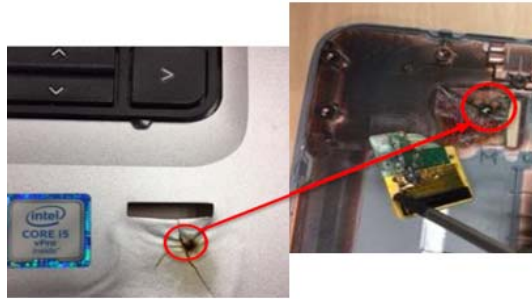
Plastic keyboard deck burnt photo
