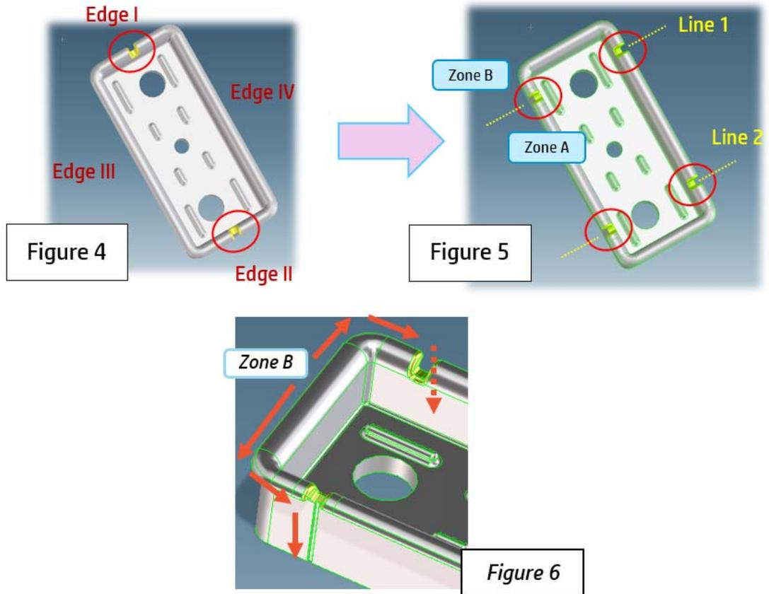
An additional advantage of the proposed four notch design, such as shown in Figure 5, is that by having four notches (rather than just two) there is a decreased likelihood of notch blockage (e.g., by ink drool).
