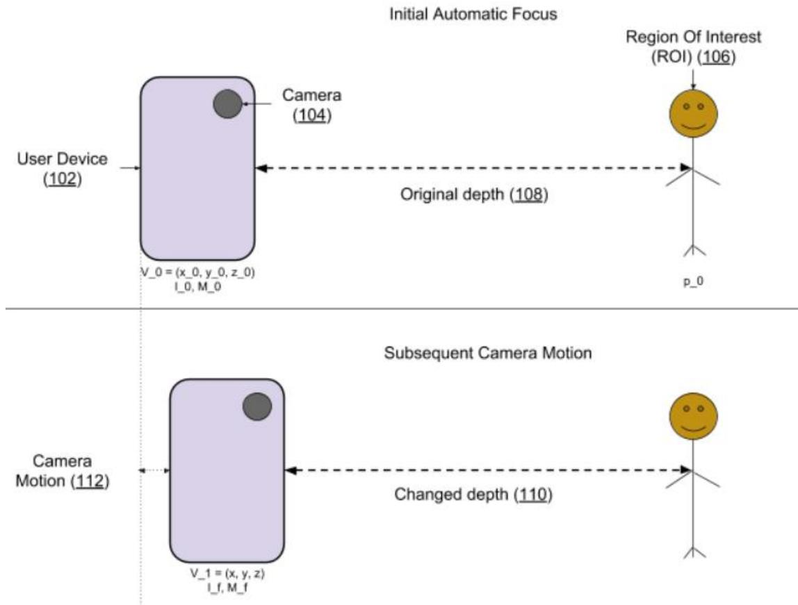
**Fig. 1: Triggering adjustment to automatic focus to compensate for camera motion**
