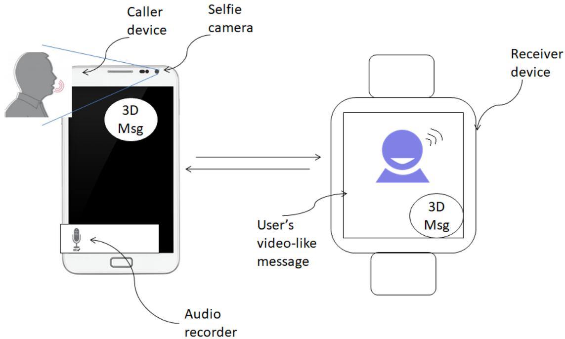
FIG. 1: System to send and receive video-like messages
