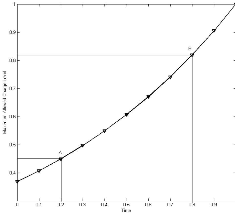
**Fig. 1: Maximum permissible charge level as a function of time since last recharge**
