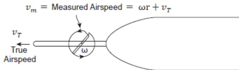
FIG. 4: Airspeed measurement device showing true airspeed and measured airspeed
