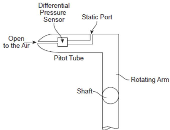
FIG. 2: Rotating pitot tube comprising a differential pressure sensor
