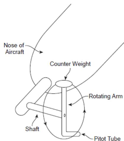
FIG. 1: Airspeed measurement device comprising a pitot tube at the end of a rotating arm
