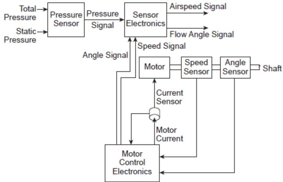
FIG. 3: Airspeed measurement device sensors and electronics
