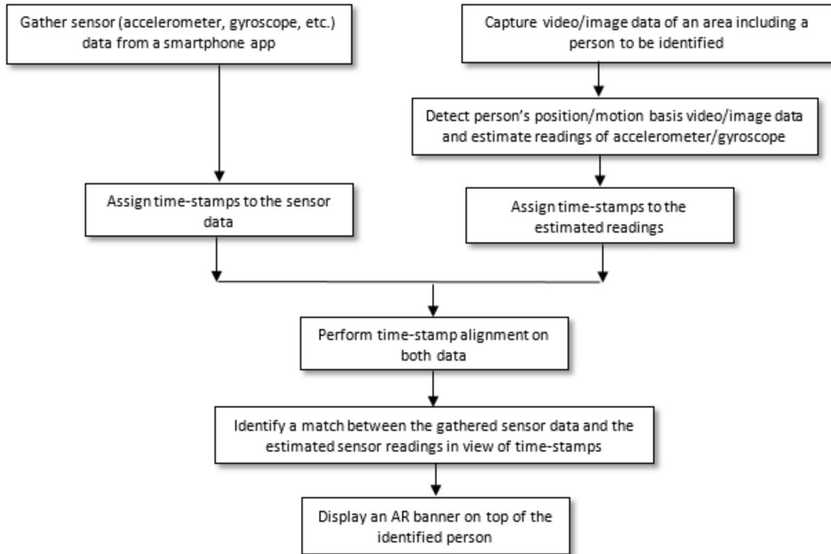
Figure 1: Block diagram for displaying an AR banner
