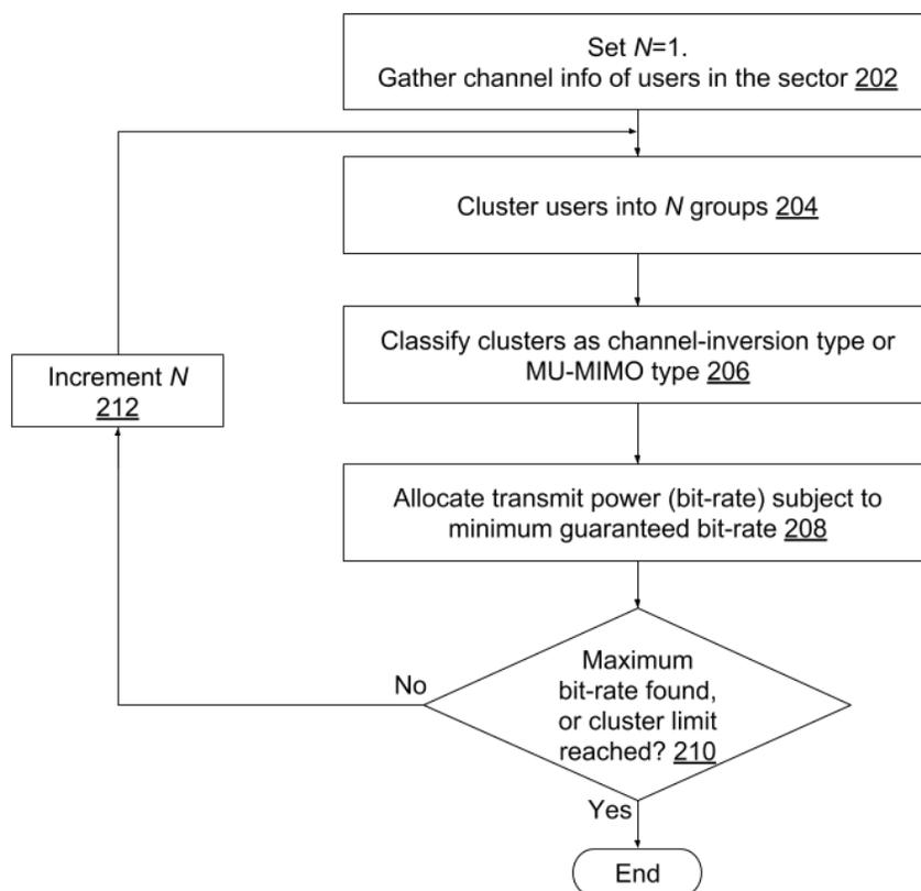
**Fig. 2: Optimizing aggregate multicast bit-rate subject to a minimum guaranteed per-user bit-rate**
