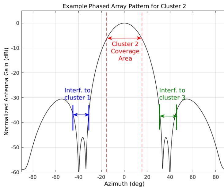
**Fig. 5: Radiation pattern of a phased array that is targeting RF energy at cluster 2 (near zero degrees azimuth) while minimizing RF energy at clusters 1 and 3 (near  $\pm 40$  degrees)**
