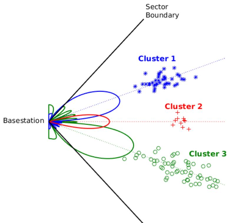
**Fig. 6: Radiation patterns resulting from the power or bit allocation procedure of this disclosure**
