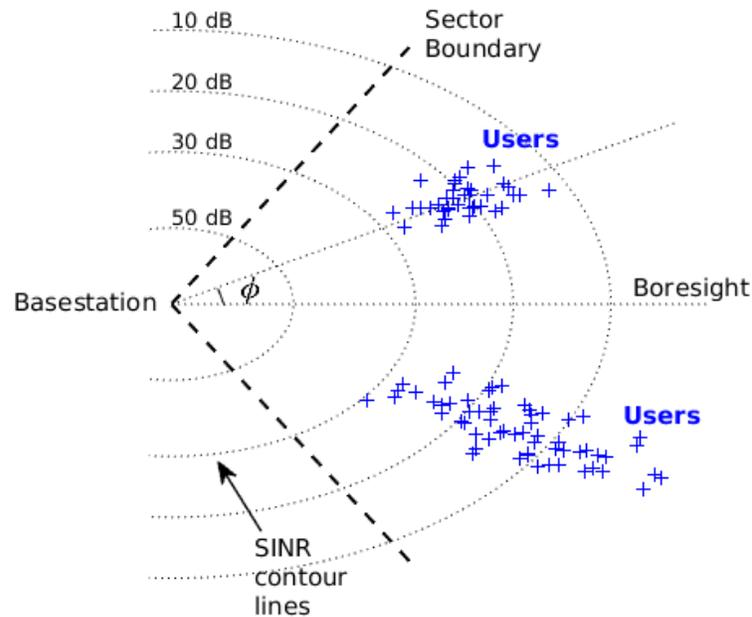
**Fig. 3: Angular ( $\phi$ ) and SINR map for multicast users in a sector**
