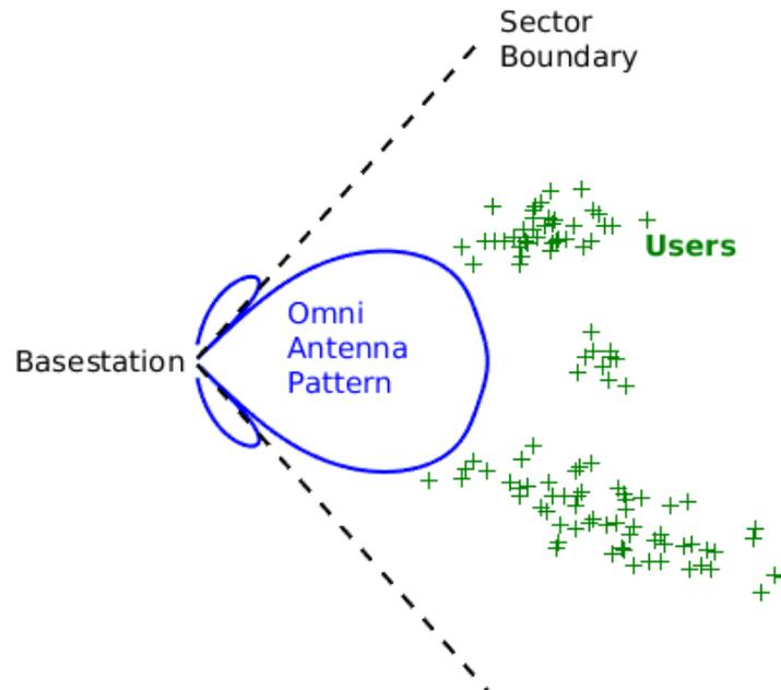
**Fig. 1: Omni-directional radiation pattern for spatially separable users is sub-optimal**
