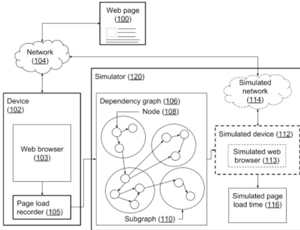
**Fig. 1: Recording web page loading on one device and simulating it for another device**
