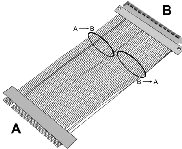
**Fig. 1: PCIe link with symmetric bidirectional bandwidth**
