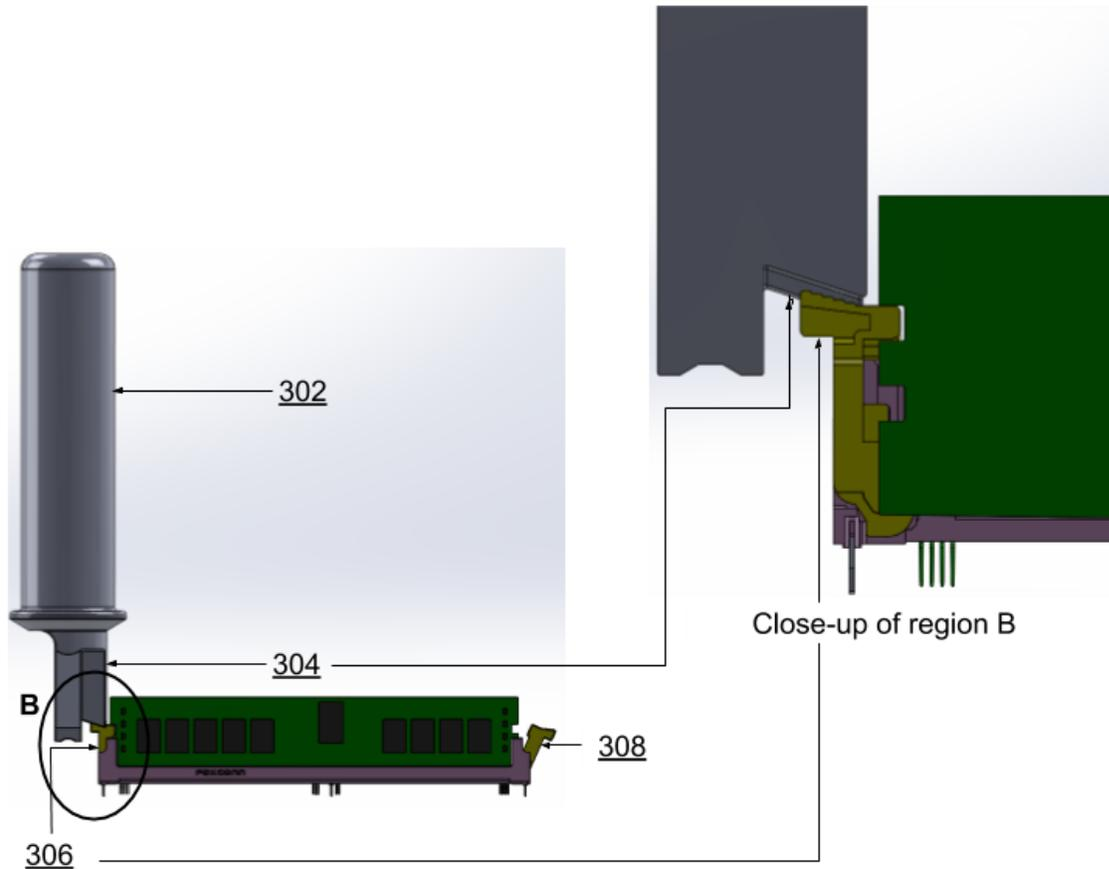
**Fig. 3: Unlatching a DIMM using the tool**
