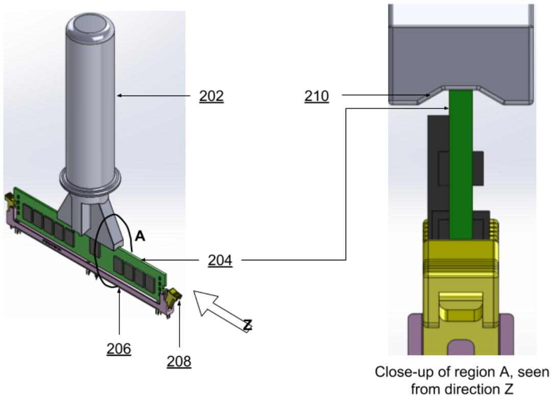
**Fig. 2: Inserting a DIMM using the tool**
