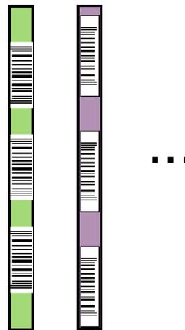
**Fig. 4: Colored and barcoded cables in one or more colors**
