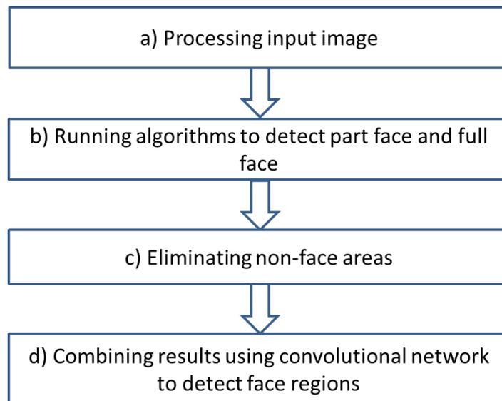
FIG. 2: Method for facial detection
