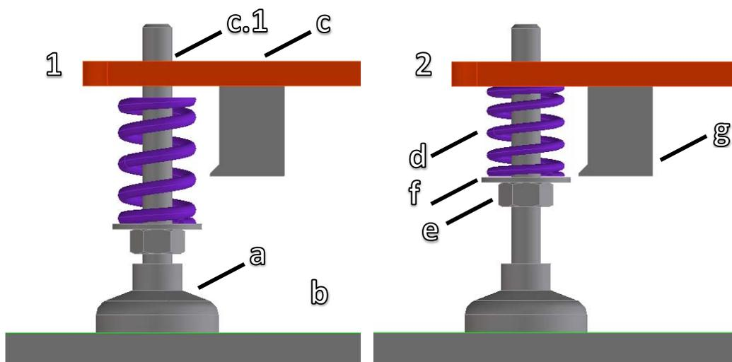
Figure 1 and 2 – Leveling foot embodiment
