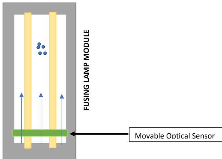
The proposed sensor is commonly used in the automotive industry as dirtiness sensor for headlights and similar than rain sensor.
