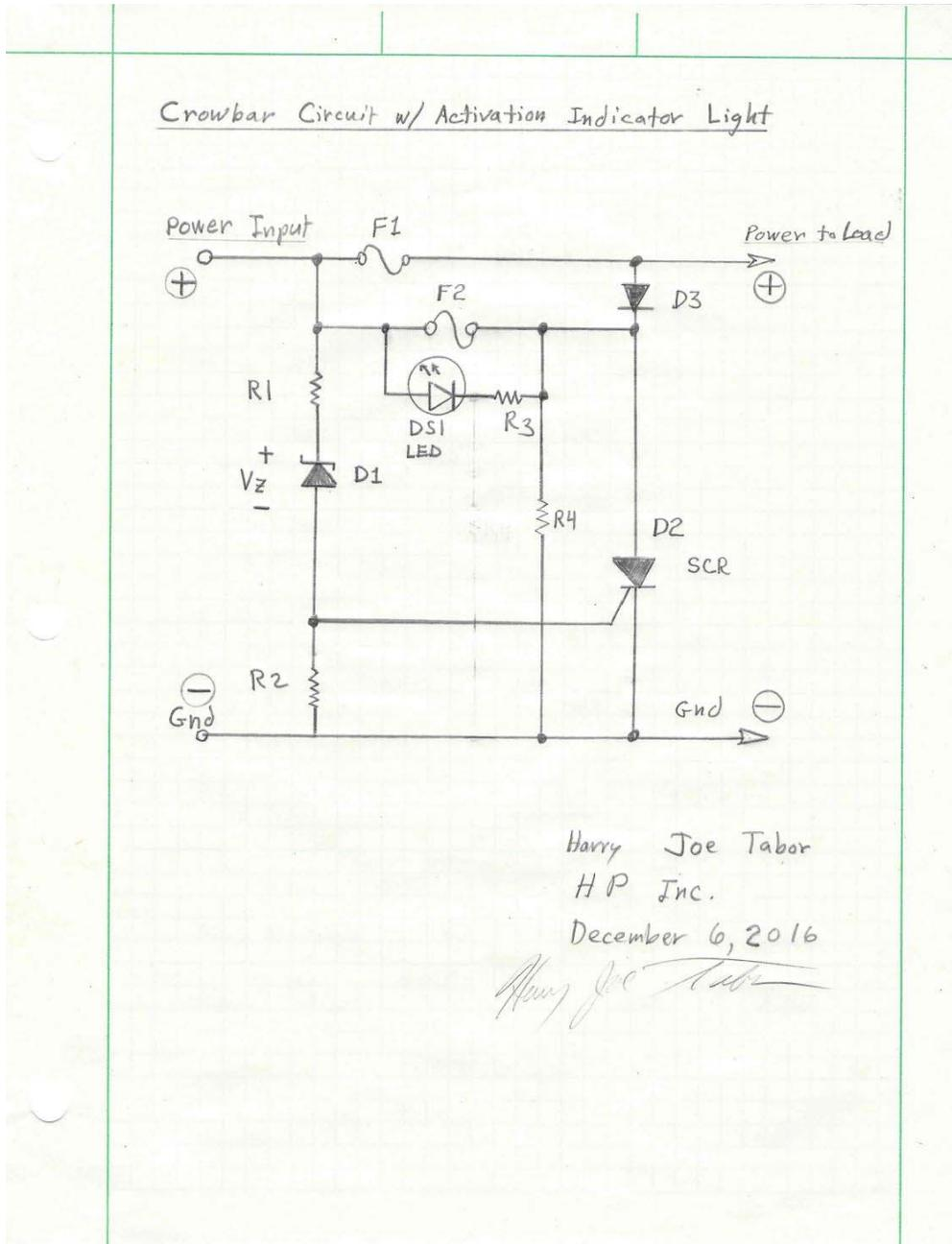
Figure 1: Crowbar Circuit with Activation Indicator Light
