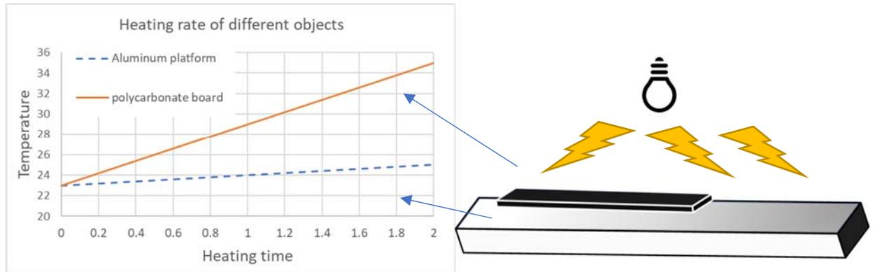
Schematic: Right: Illustration of test setup (heat source, platform and foreign object). Left: typical heating curve for a thick aluminum platform and a polycarbonate board during 2 seconds of heating.
