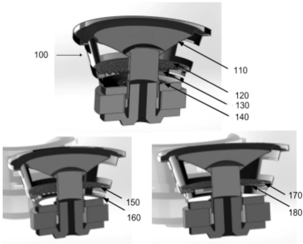
**Fig. 1: Charged electrodes attached to a moving coil transducer**
