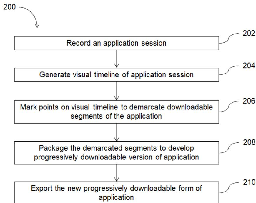
FIG. 2: A method of visually constructing a progressively downloadable application
