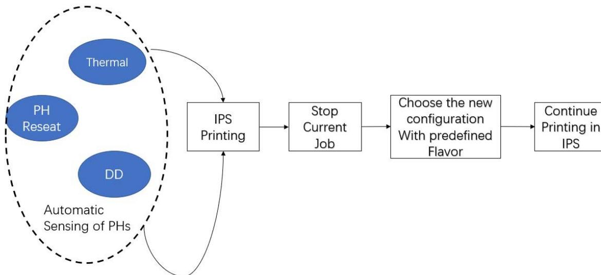
Figure 3 Automatic adaption workflow during printing
