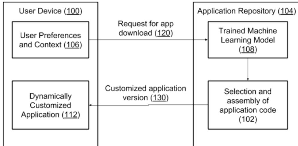
**Fig. 1: Customized dynamic delivery of a software application**
