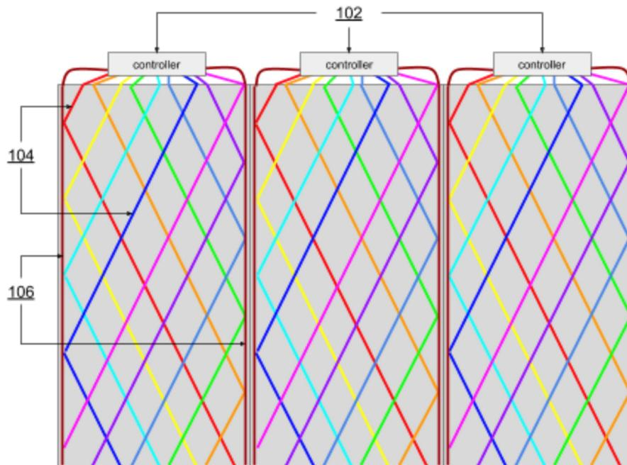
**Fig. 1: Segmented large-scale touch / proximity sensor**
