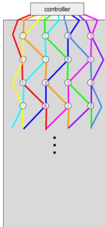
**Fig. 2: Alternate wiring pattern for segmented large-scale touch / proximity sensor**
