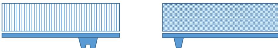
Figure 2 – different supporting heatsink with just one contact point (“one foot”)
