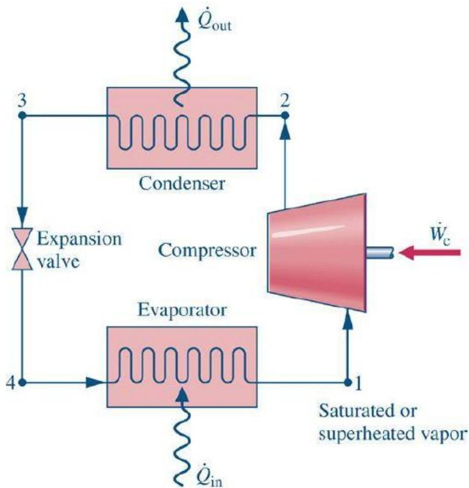
FIG. 1 – Conventional cooling cycle
