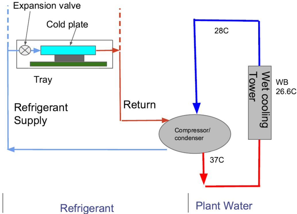
FIG. 2 – New thermal architecture
