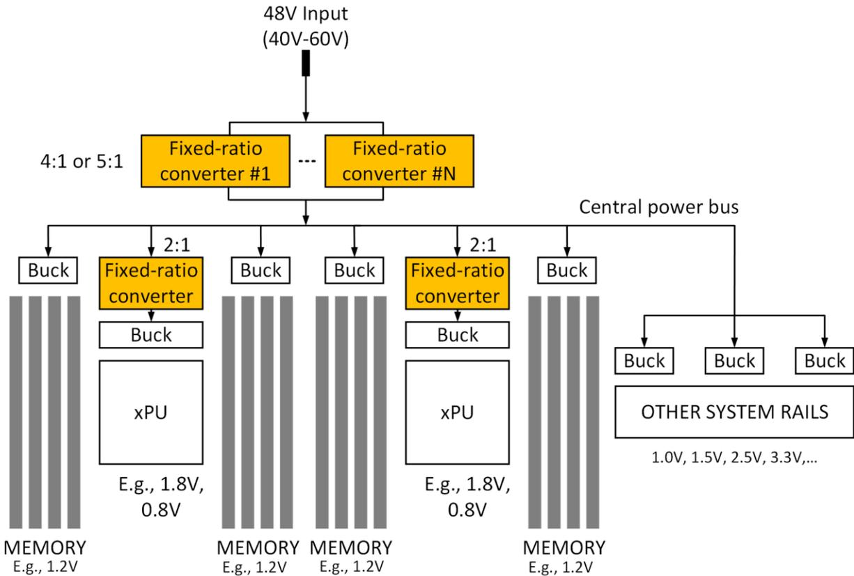
FIG 1. Multi-stage 48V-to-PoL power architecture for ultra-high current xPU applications
