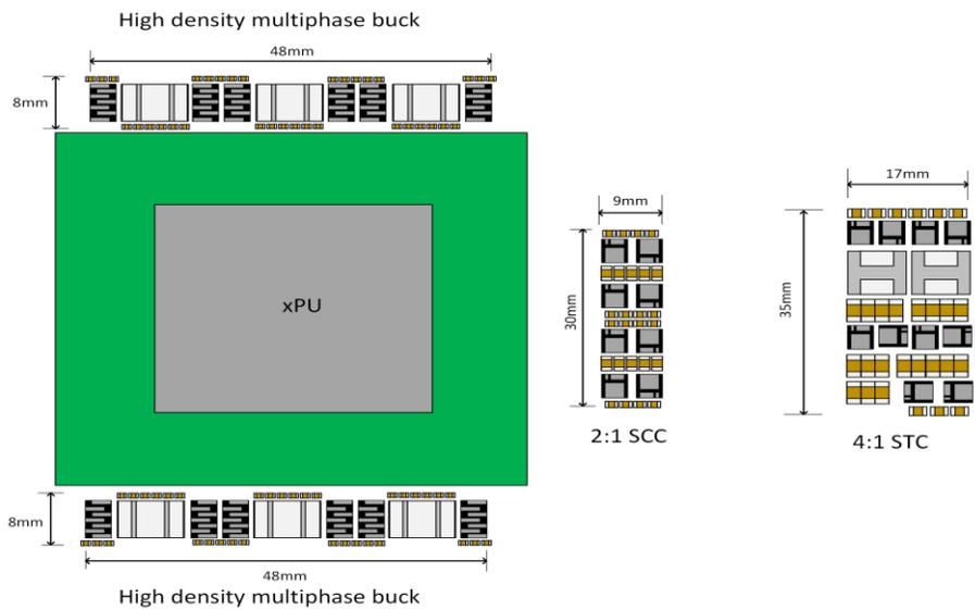
FIG 4. Physical layout of the multi-stage 48V-to-PoL power architecture
