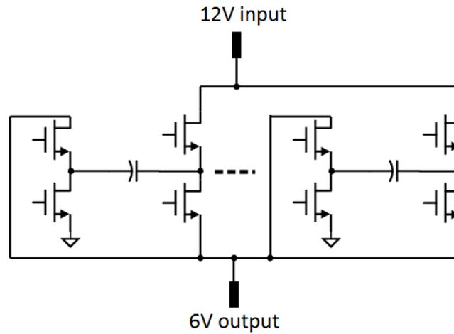
FIG. 3 Example second-stage fixed-ratio converter: a multi-phase 2:1 SCC fixed ratio converter
