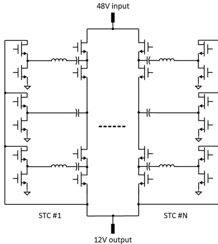
FIG. 2 Example first-stage fixed-ratio converter: a multi-phase 4:1 STC fixed ratio converter
